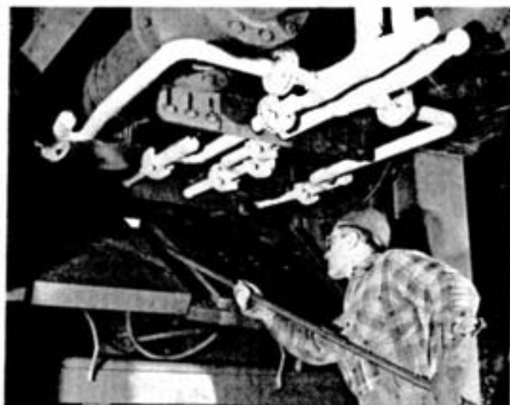
AT THE BURNER END of the furnace slagchute man Enio Dodda is clearing slag accretions from beneath the oxygen lances to ensure the free flow of oxygen into the furnace.
