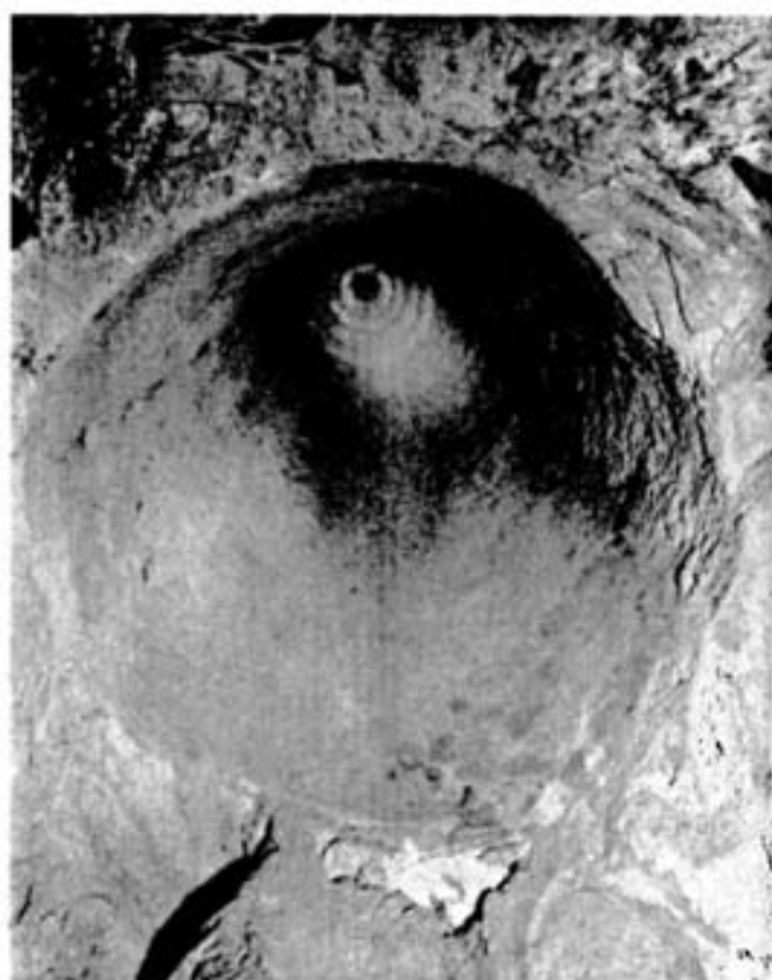
Looking up a 4-foot raise drilled by the new machine at Creighton, showing the pilot hole and pattern of the cutters.
