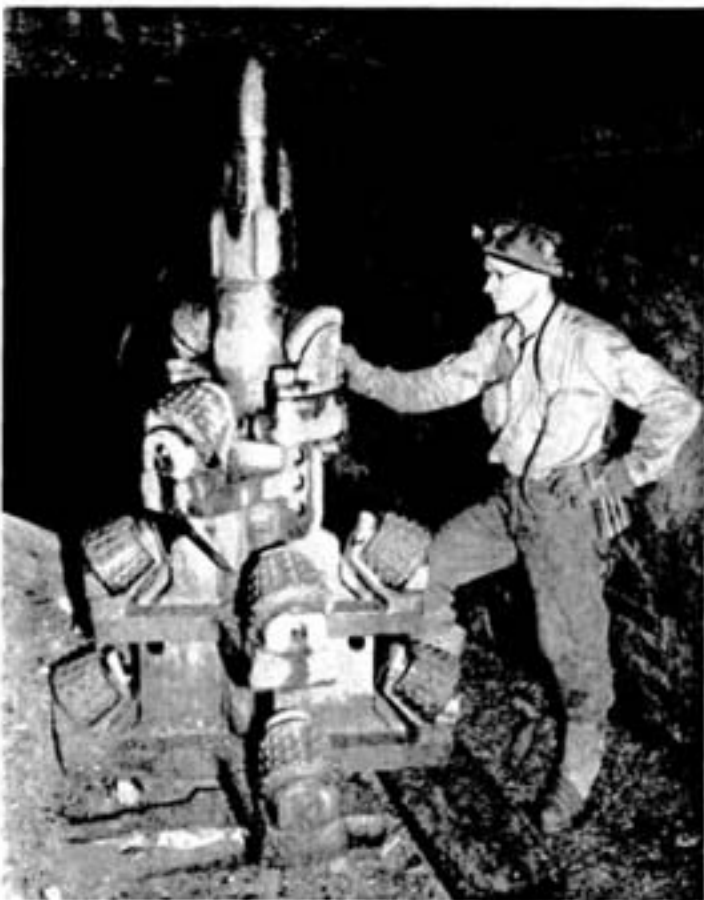
This reaming head, which enlarges a 9½-inch pilot hole to four feet, has 12 tungsten-carbide cutters.
