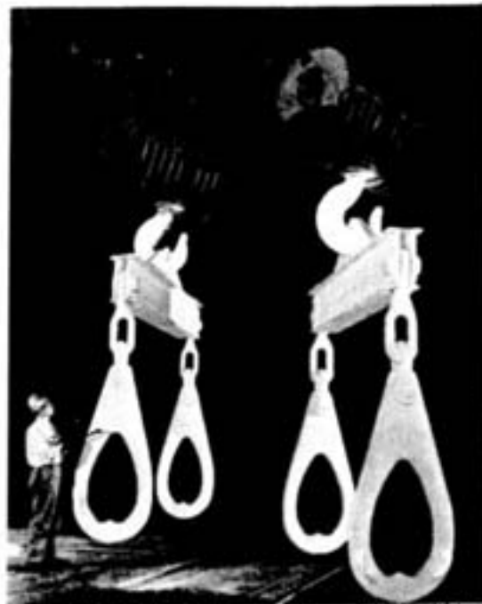
AT THE BEGINNING of each 8-hour shift the lifting bails on the cranes are inspected and the lower end of the hoist assembly checked for freedom of movement. Wielding the testing hammer in the picture is Pat Weir.
