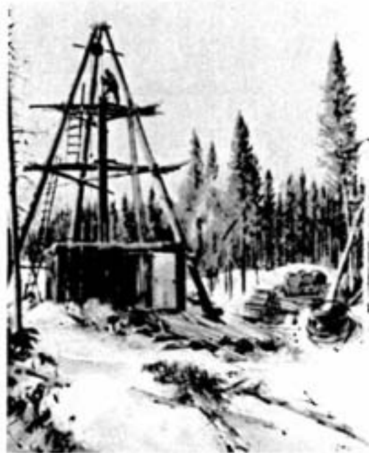
Diamond Drill Rig in the Manitoba Bush near Thompson.
