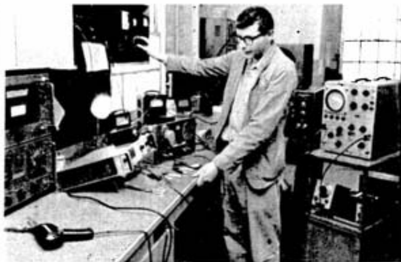
company to build and use this device to search for ore deposits. 2. Of great importance to an exploration crew "in the field", both for efficiency and safety, is dependable radio communication. Here technician Doug Stickles is measuring the frequency of a radio unit that will accompany a summer exploration team to Northwestern Ontario.
