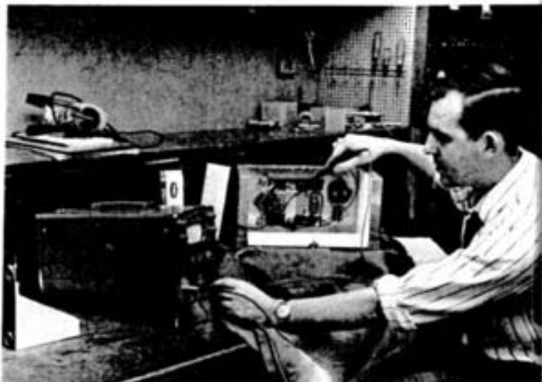
determine the direction of the electro-magnetic field set up by the transmitter and also a secondary field induced by the presence of sulphides or another electrical conductor; technologist Bob Williams is shown in this picture testing the frequency response of a pickup or receiver coil.
