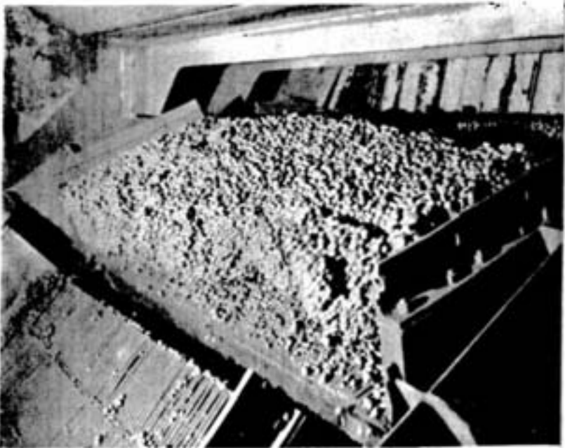
IRON ORE PELLETS, fired at a temperature of 2400 degrees F., come off the traveling grate machine, after being dried, fired and finally cooled.
