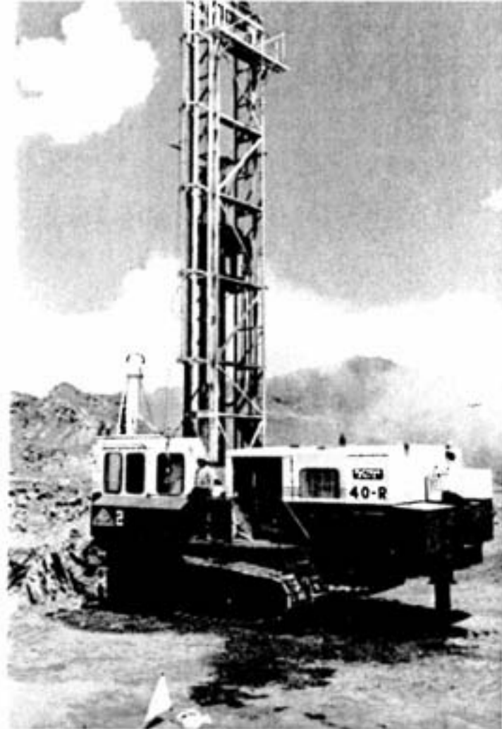
One of Clarabelle's two new rotary drills which have put 10 old-style churn drills out of business. The rotary drill cuts a 9-inch hole at the rate of 130 feet per shift as compared with the churn drill's average of 18 feet per shift. It has a down pressure capacity of 45,000 pounds, and can drill a hole 90 feet deep, ejecting the cuttings with compressed air. It weighs 40 tons, and is 48 feet to the top of its derrick.
