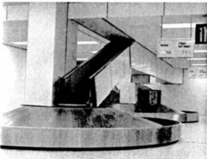
The baggage carousels, subjected to hard usage, will remain brightly new on account of their nickel stainless steel construction.
