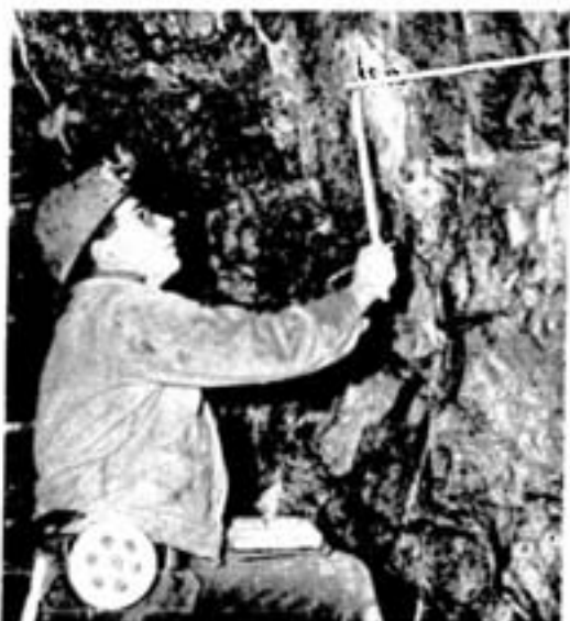
Garry Klein is taking an ore sample after first marking up the ore contact in 38.5 stope on 1400 level. Marking the ore contact is standard procedure by the geologist to assist in the efficient mining of the irregular Thompson orebody. The sample Garry is collecting will be taken to the geological department for visual estimates of its metal content and may then go on to the laboratory for assay.
