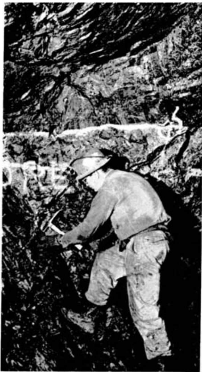
Garry Klein is taking an ore sample after first marking up the ore contact in 38.5 stope on 1400 level. Marking the ore contact is standard procedure by the geologist to assist in the efficient mining of the irregular Thompson orebody. The sample Garry is collecting will be taken to the geological department for visual estimates of its metal content and may then go on to the laboratory for assay.
