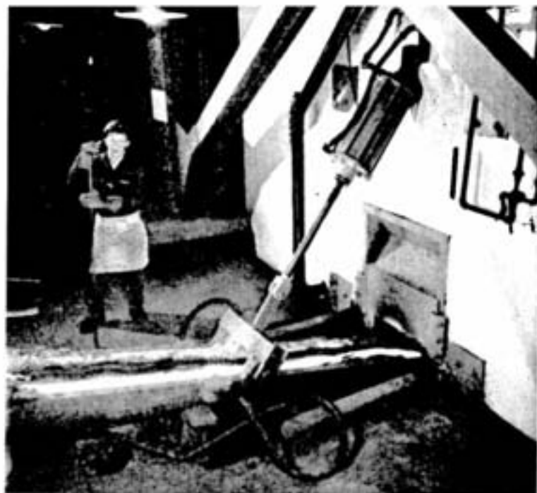
This is the slag skimming setup at each of Thompson smelter's three electric furnaces, showing the water-cooled launder, granulator pit, and air-operated safety device for diverting the flow of slag in the event of an emergency.
