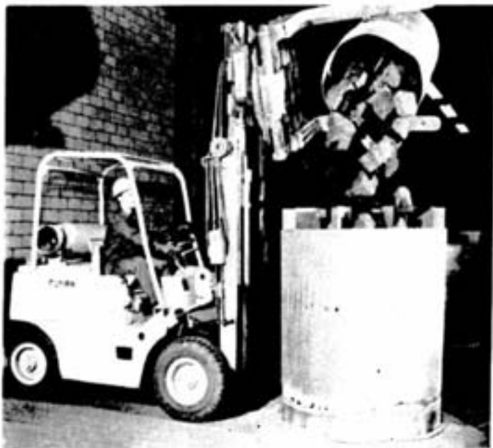
HIGH UP in the 127-foot Thompson smelter Dale Paterson is seen filling an added electrode section with chunks of carbon paste, the "mix" that melts and then bakes into a solid cake as it is gradually lowered to the furnace. Jutting above the rim of the steel casing are the fins which add support and conductivity to the electrode.
