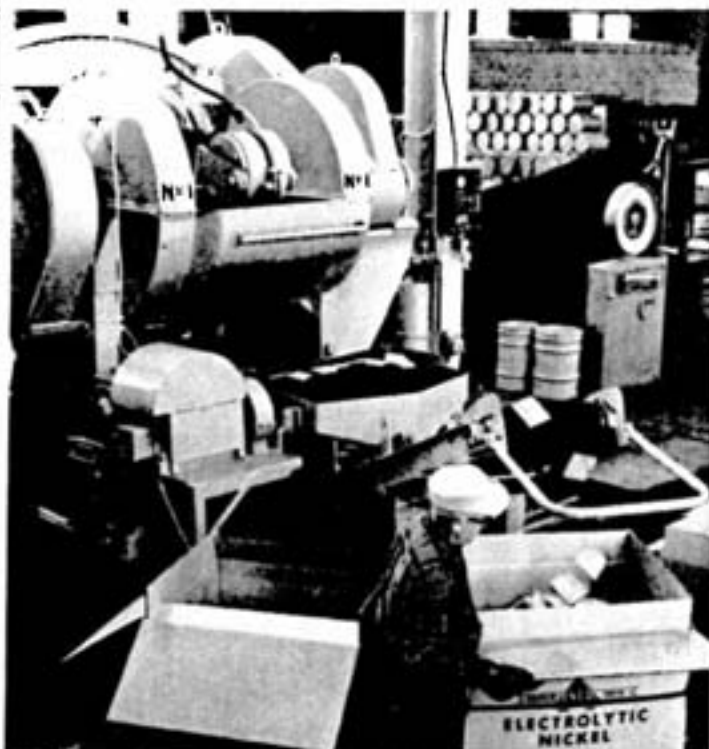
3. On the other side of the shears the squares of nickel are picked up by a conveyor and loaded into double-walled fibre boxes, one of several types of containers in which Inco Nickel goes to market. Ed Gravelle is checking the squares for appearance and shape as they come tumbling off the conveyor belt.
