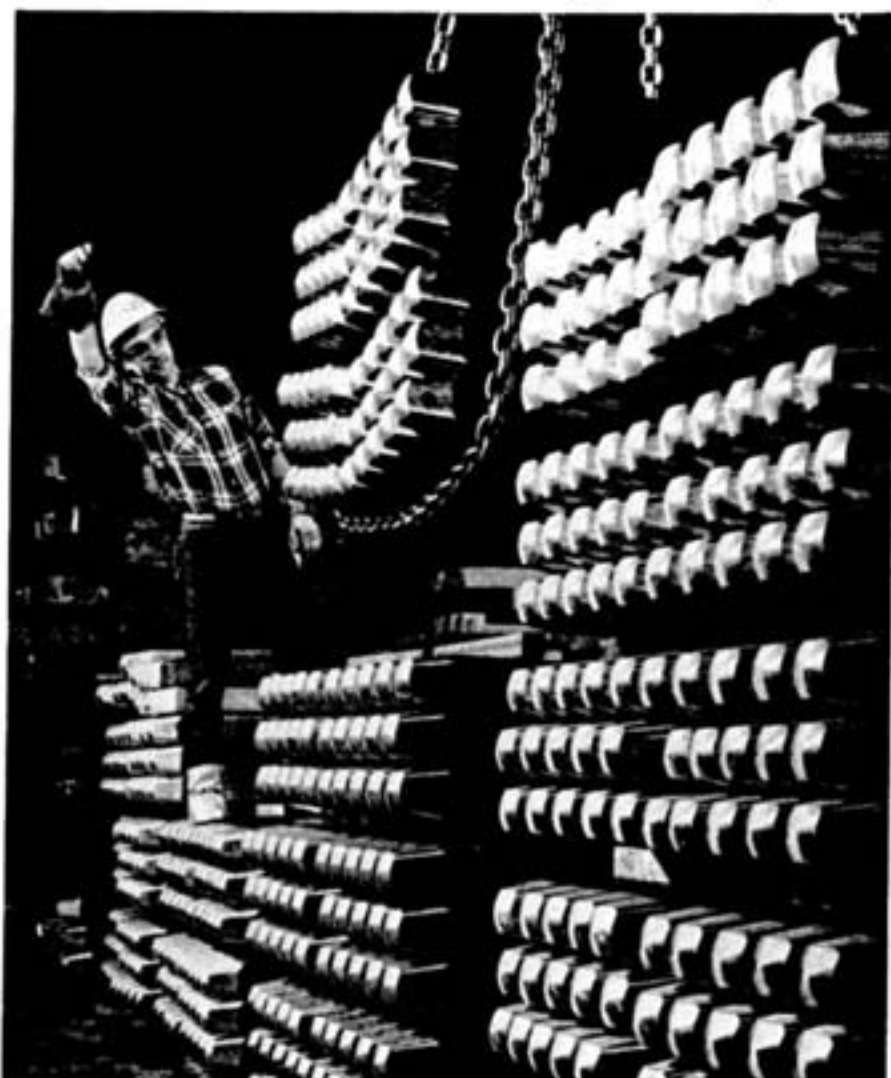
The glowing coppery snouts of machine-tapered wire bars, stacked tier upon tier, offer an irresistible pattern picture to the photographer at large in the Copper Refinery. George Hunter, the Toronto camera artist, made this dramatic, clean-cut portrait of man and metal as crane follower Nordfried Locke signals the crane in placing a lift of the vertically cast bars in storage. One of over 60 special vertically cast copper shapes produced at the Copper Refinery, this bar has superior qualities which make it particularly desirable for the production of high grade rod and wire.
