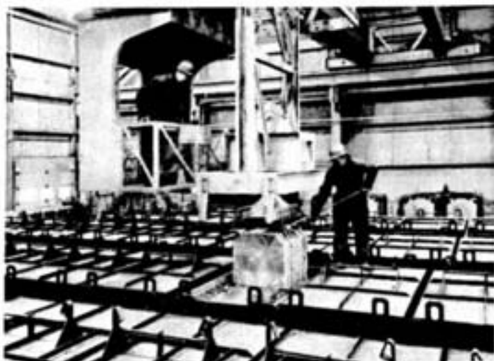
In the top photograph Leo Bremner is shown operating the box crane, lifting anodes from one of the big annealing boxes for shipment to the tankhouse in the refinery. Below is a closeup of the ladle car as it pours a 475-lb. anode into one of the row of moulds. The ladle holds 4 tons of molten bessemer matte, which is poured onto an attached diffuser to spread it over the mould. The operator shown is Emile Romain.
