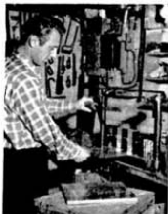
He designed and made the equipment to mass-produce his lunch buckets. Here he drills rivet holes in a batch of blanks.
