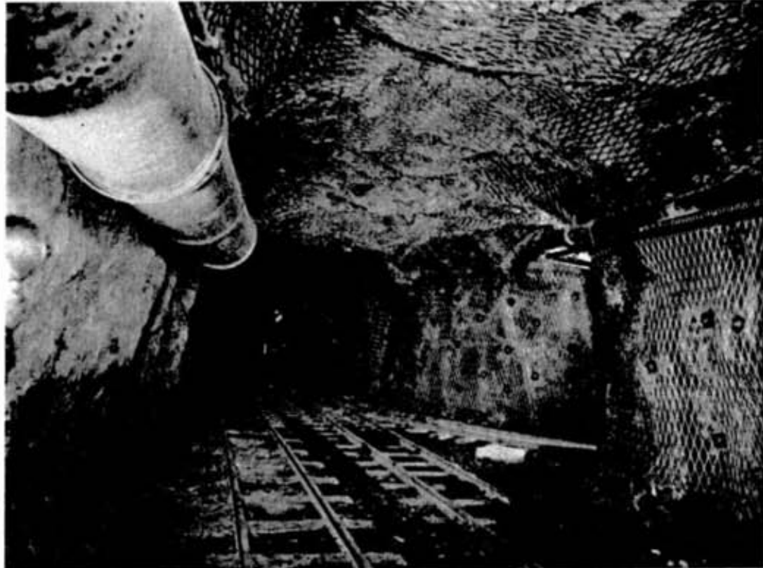
Screenbolting is particularly effective in wider areas of the underground workings such as this intersection on 6200 level at Creighton's no. 8 shaft. Shift boss Ray Allison is seen checking the installation.
