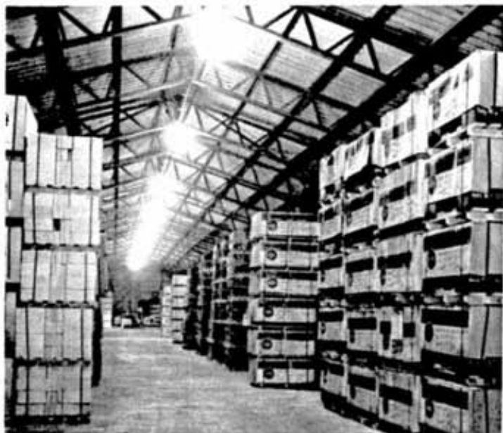
Interior view of the new refractory warehouse at Copper Cliff. Handling of material is now greatly facilitated with all brick received in pallet form. RIGHT: One fork lift truck easily handles all incoming and
