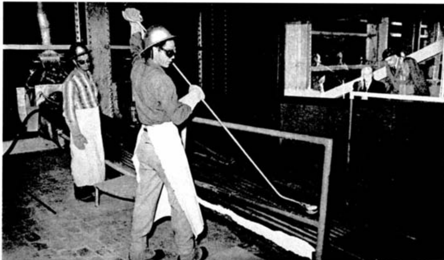
On his visit to Copper Cliff smelter the Governor General saw nickel matte being tapped from a reverberatory furnace. Here he is seated behind a glass screen, while reduction plants manager R. R. Saddington describes the operation. The furnacemen in the foreground are G.
