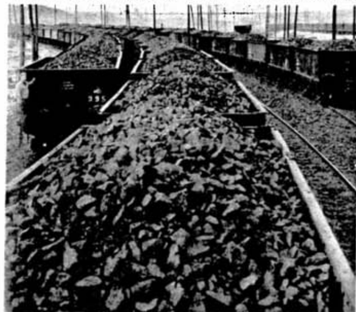
Part of the ore storage area near the Copper Cliff crushing plant is shown here. A train of ore cars is about to be pushed up the incline to the receiving bins at the crushing plant.
