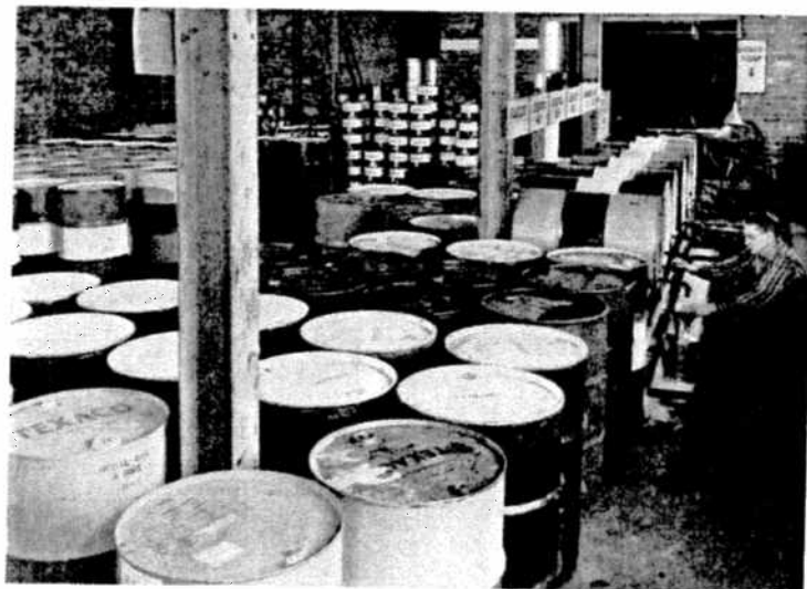
Part of the oil house, separated by a brick wall and fire door, is shown here. Oil, grease, kerosene, naptha, lysol, liquid soap and drums of paint are stored here. Henry Nelson is drawing off a can of oil.
