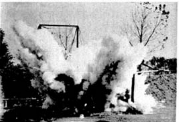
TO DESTRUCTION. The cylindrical tank did not burst until it had been subjected to the terrific internal pressure of 2,160 pounds per square inch. Flying fragments are not steel but insulation.
