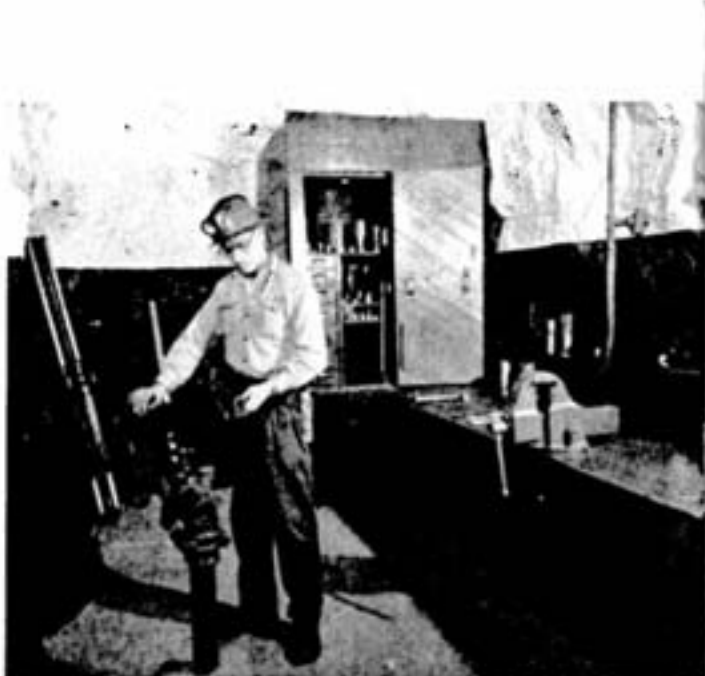
In this view of an underground steel-testing station at Frood-Stobie mine, a drilling crew is conducting a regular test of drill steel. The drillers are Leo Rivest (nearest camera) and Omer Vallee. The test engineer, Fred Horner, controls the air pressures for both machines, and times and measures each run. He also sharpens and gauges the inserts. The picture on the right shows one of the underground drill repair shops which are strategically located in each of the Inco mines; the drill fitter is Al Saulnier.
