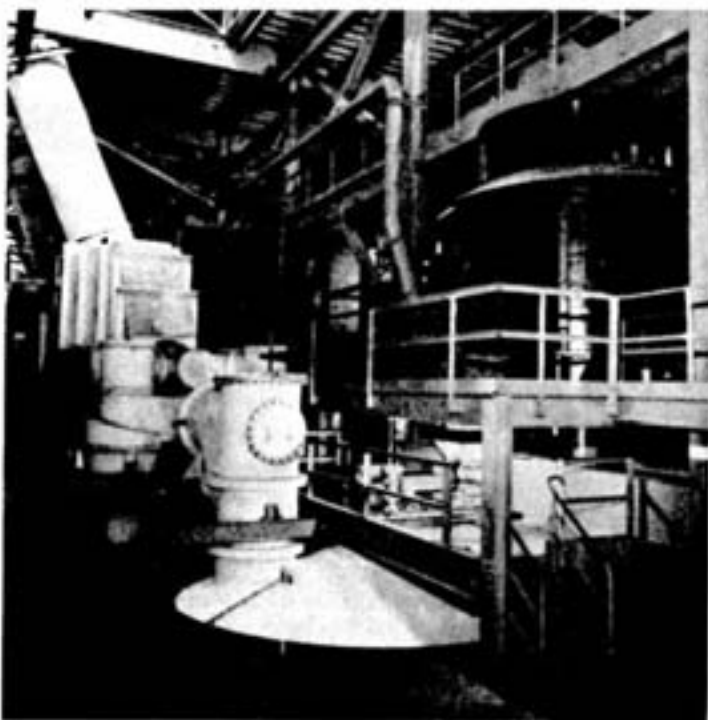
This view of the feeder floor up in the smelter shows a rotary concentrate bin on the right, the feeding mechanism and part of the conical top of the fluid bed roasters, and a calcine recovery unit. The man on the platform is Mike Bahalle.
