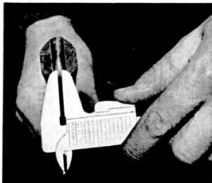
Measuring the wear of a tungsten carbide drill steel insert. Careful Inco research studies have determined the maximum dullness to which an insert should be drilled, and also the degree to which it should be sharpened to give optimum drilling performance.
