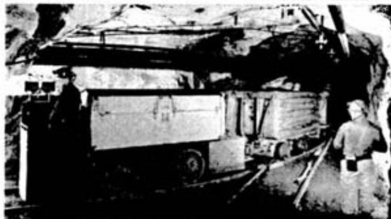
A battery locomotive and train of ore cars on 1000 level, Thompson mine. Members of the motor crew are Bill Foote, motorman, and Ferdinand Fursthaller, switchman.
