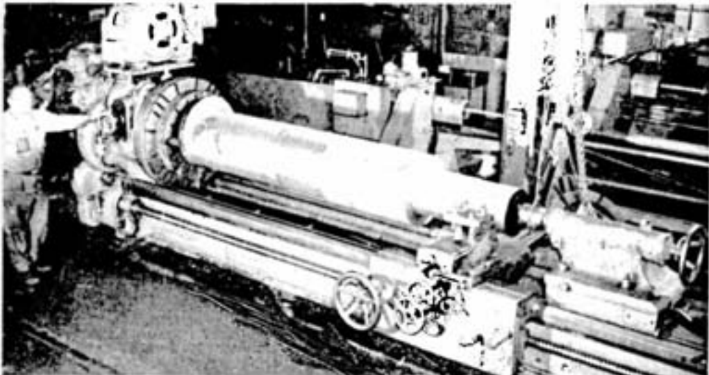
One of the biggest jobs ever handled in the machine shop was making a new shaft for a standard Symons crusher out of an old jaw crusher shaft. In the first stage of the operation Alan Butler is seen doing the rough cutting of the old shaft on his 36-inch American lathe.
