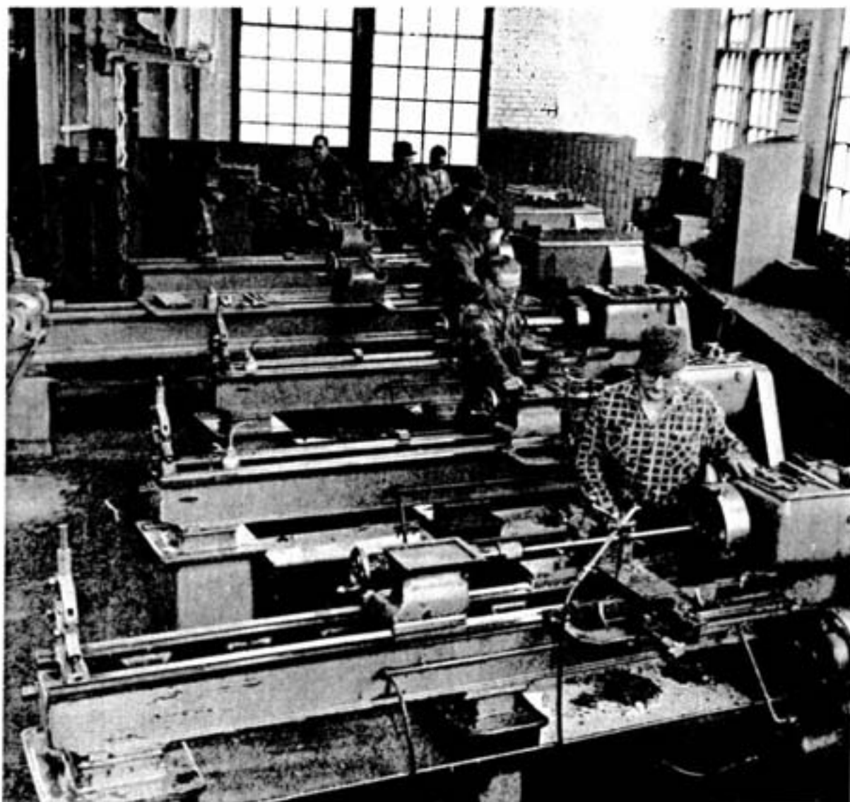
This group of seven lathes occupies one bay of the machine shop and handles a great variety of work. They turn shafts, make bushing, pinion and sprocket blanks, crusher adjusting bolts and do screw cutting on valve stems. Operating the machines from front to back are Stan Bryson, Wes Blueman, George Renaud, Owen O'Reilly, Graham Denmark, Roly Veccka and Harry O'Connell. There are 32 lathes in the shop.
