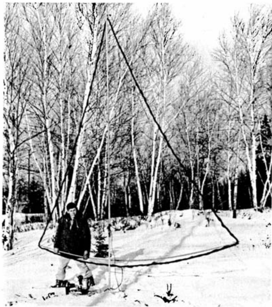
ABOVE: Doug Adolph, motor generator unit at his feet, aligns the vertical transmitting coil of the "E.M." apparatus, while Henry Levac uses the receiving coil of the "E.M." apparatus to determine if a conductive body is effecting the signal from the transmitter. LEFT: Henry Levac operates a Sharpe magnetometer. RIGHT: Bob McGregor reads a Worden gravimeter.
