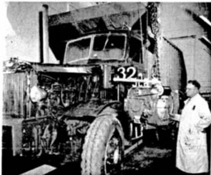
In the picture on the left the GMT-305 Whirlfire gas turbine engine is shown in comparison with an ore haulage truck like the one it will power in an extensive field test at the Open Pit. Standing beside it is J. "Buster" Dyck, assistant master mechanic of mines. On the right the revolutionary new gas turbine engine is seen on its portable stand beside one of the diesel engines regularly used in the Open Pit ore haulage trucks. The diesel job weighs 2,830 lbs., the Whirlfire 750 lbs.
