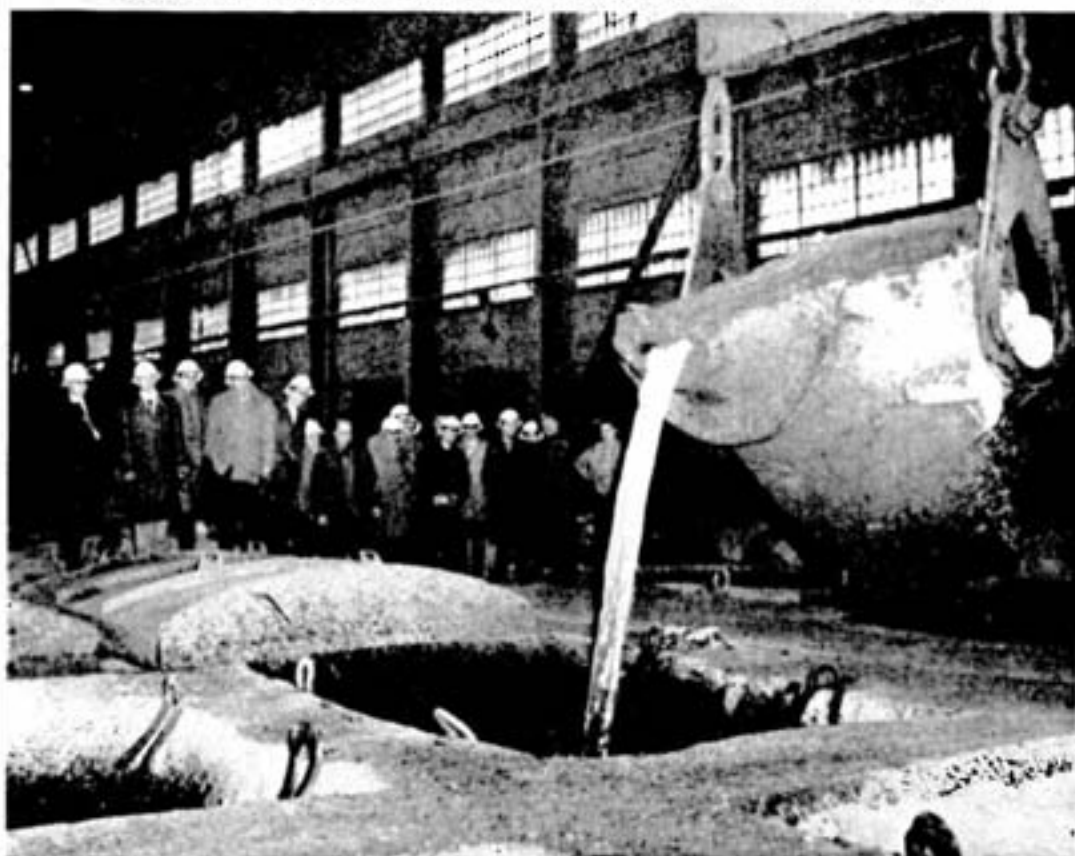
Thirty-six metallurgical students from the University of Toronto and McMaster University, Hamilton, were keenly interested visitors at Inco operations at Copper Cliff. The picture shows a group watching casting of a ladle of Bessemer matte into a mould in the first stage of the matte treatment process at the smelter; their guide is J. R. Felck, converters superintendent. Dr. H. E. Petch and Dr. W. W. Smeltzer of McMaster and H. U. Ross and A. W. Lund of the University of Toronto were the faculty members accompanying the party. At a luncheon at the Copper Cliff Club the visitors were cordially welcomed to Inco by general manager R. H. Waddington.
