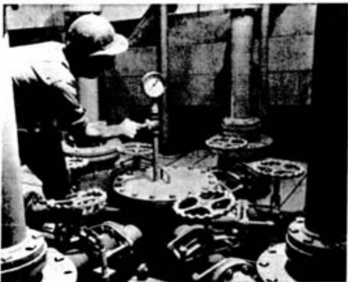
Six classifying cones are used in the production of sand fill from Levack mill tailings, and shown above is the cluster of valves controlling the cones. The gauge registers the pressure in the manifold.
