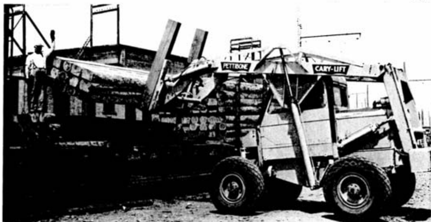
In this view at Frood mine a fork-lift truck is unloading a carload of flattened 11-foot by 8-inch mine timber and transferring it to a storage pile.
