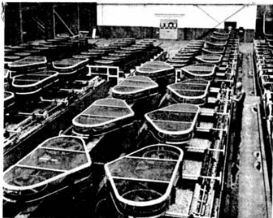
As at Copper Cliff, the mill's flotation section, partly shown here, produces a nickel concentrate and a copper concentrate. There are 50 Denver and 50 Fagergren cells in the rougher-scavenger circuit and 40 Denver cells as separators, cleaners, and recleaners.
