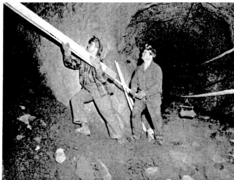
Blasting boss Cleo Gosselin and slusherman Bob Johnson demonstrate for the Triangle camera how they use the new sectional plastic tube to place powder for a blast in a hung-up boxhole in a slusher drift at Creighton no. 3 shaft. The sectional loading sticks are made of the same light plastic material as the tube.
