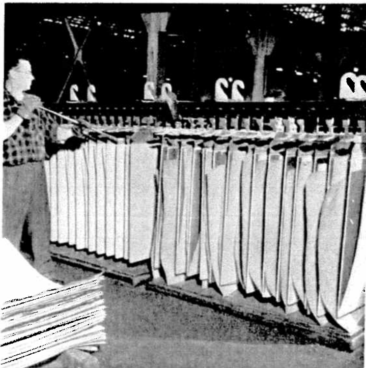
In this picture Mike Milosovic is seen stripping starting sheets from the blanks on which they were plated during a 24-hour period in an electrolytic tank. The stripper works fast, first loosening a corner of the sheet from the blank and then stripping it off with a wooden paddle.
