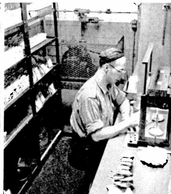
In this view of the grinding room Rolly Miron feeds ore samples to the Denver crusher and Hector Robidoux pours a partly crushed sample into the rolls. On the right Bert Potvin is making up composite samples of materials used in the plant which have been brought in for analysis.
