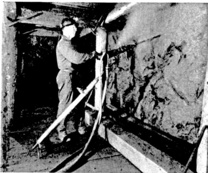
Operating an airleg drill at Frood-Stobie No. 3 shaft is Jan Szolka. He is drilling off a breast in 19.25 stope on 1400 level. Note the clean, uncluttered work area and the bulkhead in front of the driller's feet, standard safety practise at Inco mines.
