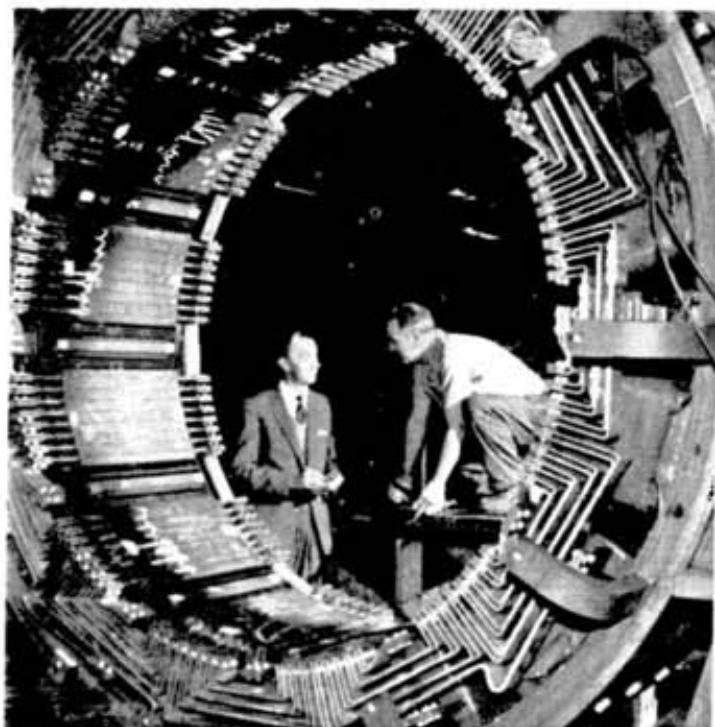
LEFT: B. J. Hayden, editor of publications at Inco's Toronto office, is seen through the stator of a big d.c. motor under construction at the Hamilton plant of Canadian Westinghouse Electric, as he covers a story for Inco Copper News. RIGHT: Mary McLeod arranges a display of a few of the items on Inco's literature list, including a copy of the latest booklet, "The Exciting Story of Nickel."
