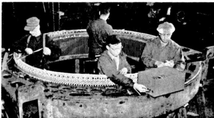
Rewinding a compressor motor for Thompson, Manitoba, are from the left, Bill Fex, Curly Tomassini, Howie Thompson and Herk Flynn.
