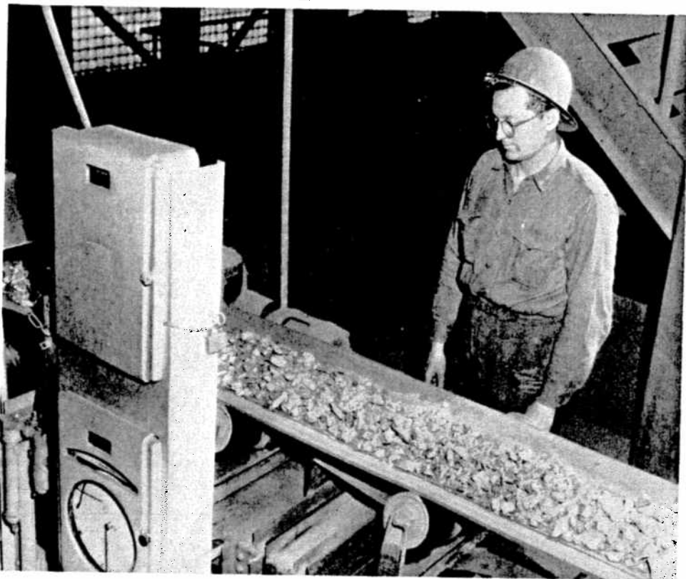
Rich in crystals of copper and nickel sulphides, now clearly defined through the metallurgical magic of controlled cooling, the gleaming matte arrives by conveyor at the grinding section of the separation department. Don Giommi is seen checking the feed to one of the rod mills.
