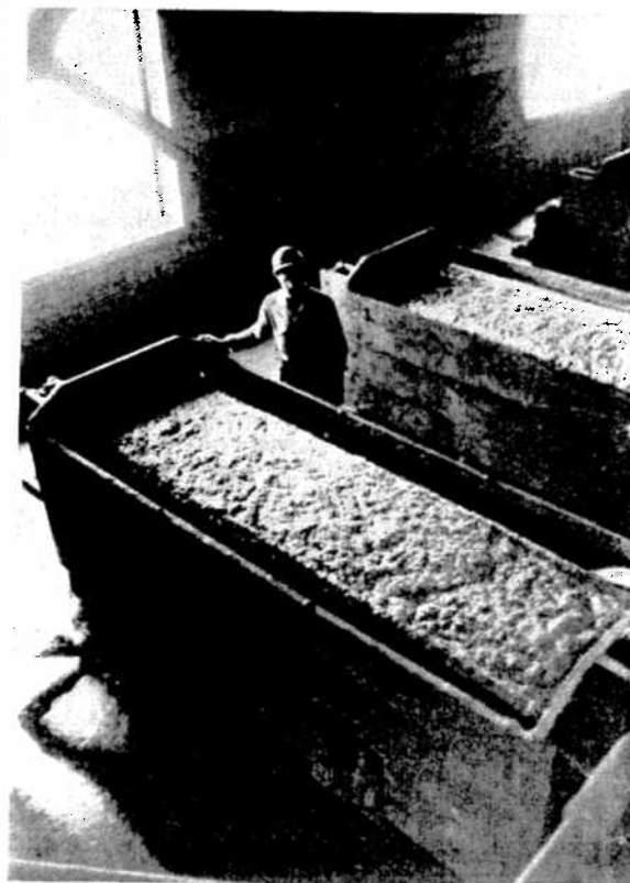
For the final stages of flotation another type of machine is used. This is a large tank in which the bubbles bearing the copper sulphide particles are floated to the surface by the agitation of the pulp. Air is introduced into the tank through a rotor covered with a rubber blade. Rheal Simard is the flotation operator helper.
