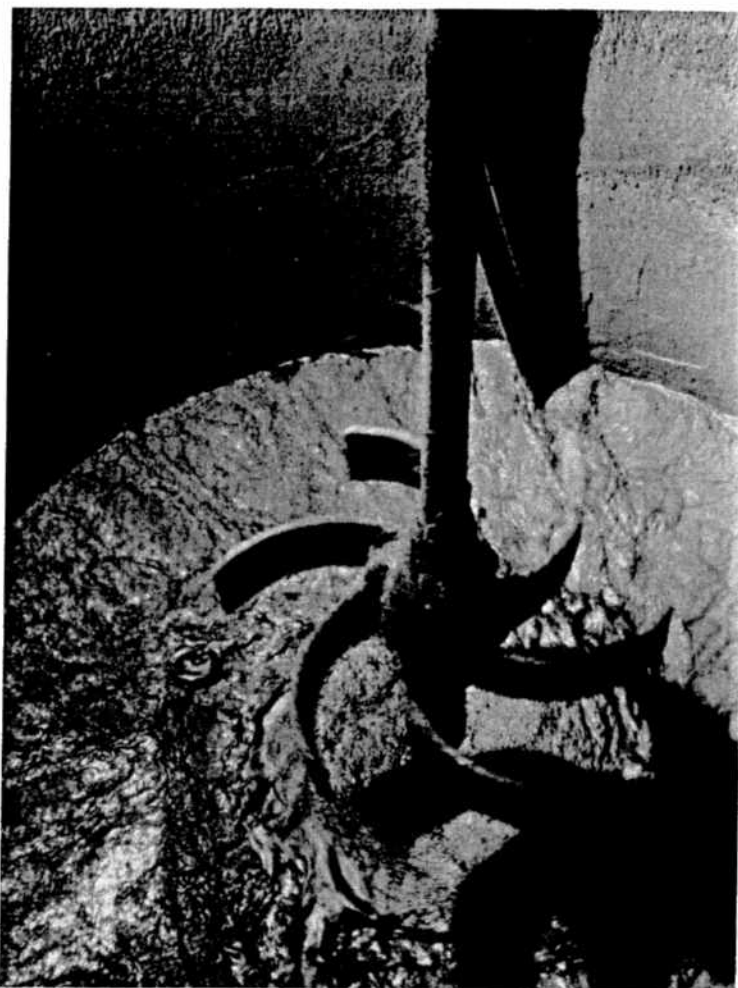
This tasty-looking brew is nickel sulphide, marking time in a storage tank before being pumped to the sinter plant for the final treatment in nickel production operations at Copper Cliff. The sinter is shipped directly to market or to the Company's plants at Port Colborne, Huntington or Clydach.
