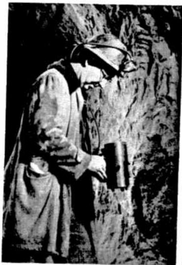
On the level 200 feet below, Art Hughes operates the coil that picks up impulses broadcast by the transmitter in the drill hole.
