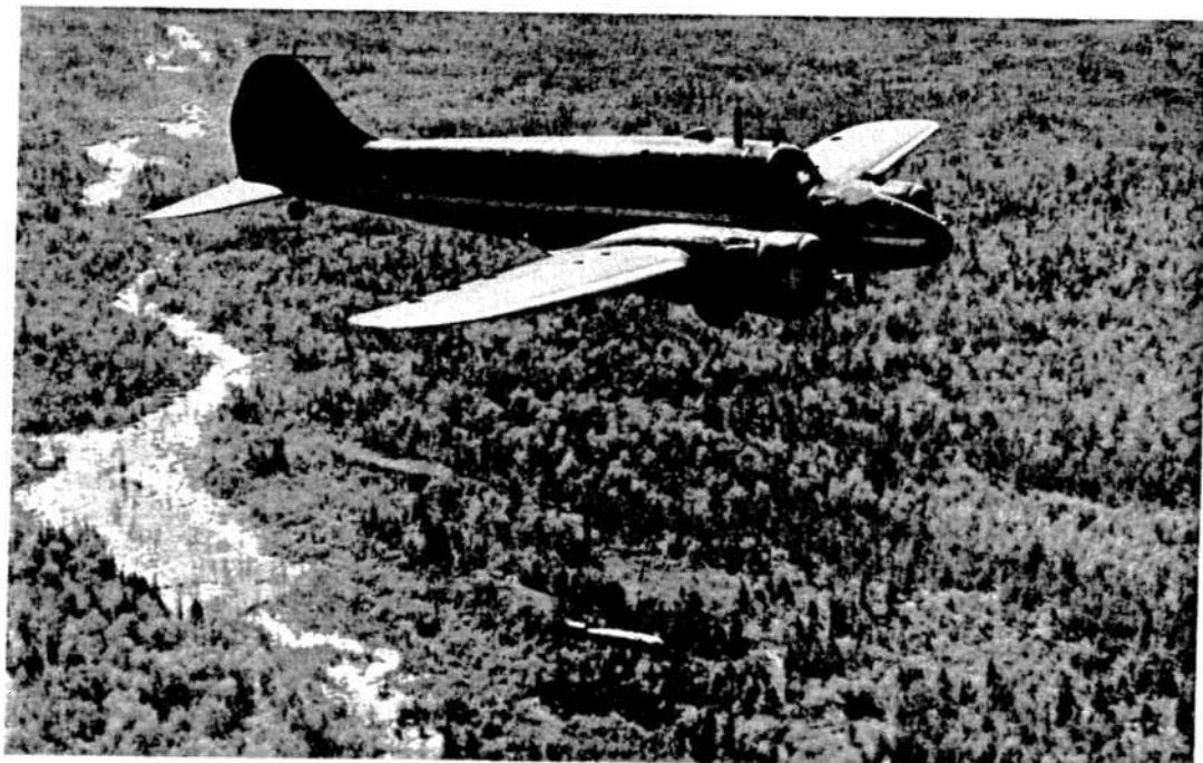
In the picture on the left the fully assembled bomb is just about ready for delivery. On the right a bomb is shown in action, towed by an aircraft over an area which is being investigated as a potential source of nickel ore. Sensitive electronic devices installed in the "flying doodle-bug" and in the plane make a record of anomalies in the ground over which they travel, and this is studied by the geological department for indications warranting more detailed investigation by ground parties.
