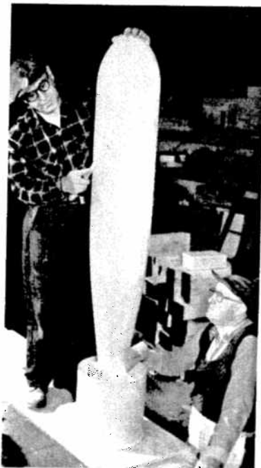
In the picture on the left the fully assembled bomb is just about ready for delivery. On the right a bomb is shown in action, towed by an aircraft over an area which is being investigated as a potential source of nickel ore. Sensitive electronic devices installed in the "flying doodle-bug" and in the plane make a record of anomalies in the ground over which they travel, and this is studied by the geological department for indications warranting more detailed investigation by ground parties.
