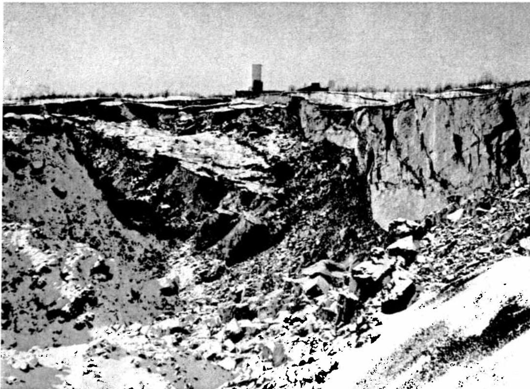
Here again winter draws a sharp picture at Creighton, clearly outlining progress in the caving operations as seen on surface. Looking across the open pit, plainly visible are the cracks and subsidence due to the orderly schedule of undercutting and withdrawal of ore going on hundreds of feet below. The cracks in the vertical face of the block on the right show how fragmentation takes place as the ore subsidizes, resulting in a large saving in blasting. Rounding out the romance of Creighton is this turn in the cycle of operations whereby the old open pit which provided the first access to the ore over half a century ago, now plays a key part in a great modern bulk mining activity. The headframe in the distance is Creighton No. 5 shaft.
