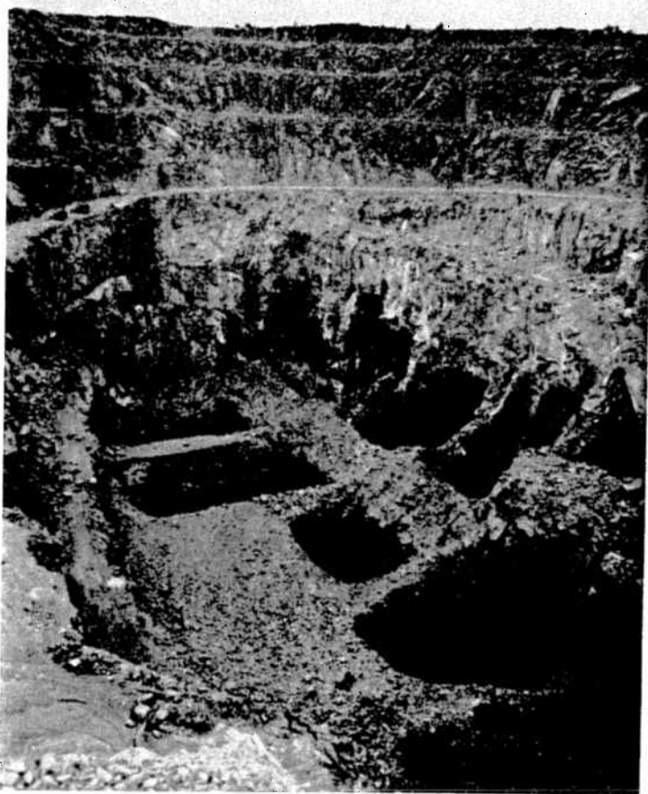
Blasthole stopes are being mined through from underground to the bottom of the Stobie section of the open pits, where surface mining was concluded in 1951.
