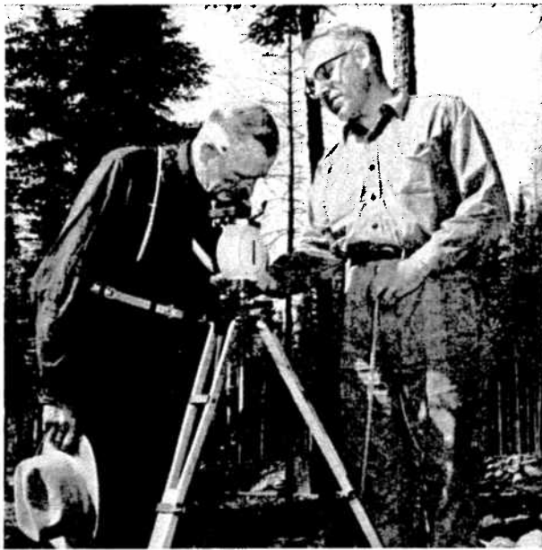
Senior physicist Herb Stewart shows M. R. Sutherland of Griswold how to take a magnetometer reading.
