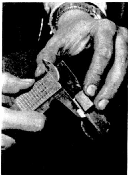
In the first of these pictures a dullness gauge is being used by the test driller to measure the amount of wear on the tungsten carbide bit insert of the steel. In the second picture test driller Vic Freelandt operates the powered grinder that sharpens the steel. In the third picture Mickey Banks, another test driller, is checking his steel preparatory to drilling. Each piece of steel in the rack is tagged and numbered so that a complete record may be kept of its behavior under test.
