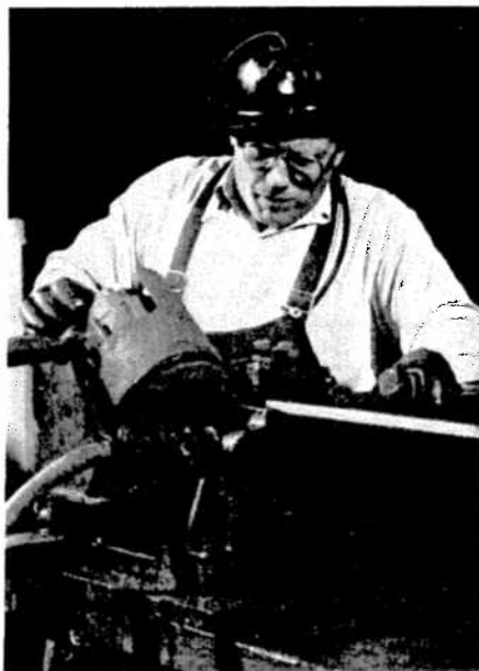
In the first of these pictures a dullness gauge is being used by the test driller to measure the amount of wear on the tungsten carbide bit insert of the steel. In the second picture test driller Vic Freelandt operates the powered grinder that sharpens the steel. In the third picture Mickey Banks, another test driller, is checking his steel preparatory to drilling. Each piece of steel in the rack is tagged and numbered so that a complete record may be kept of its behavior under test.
