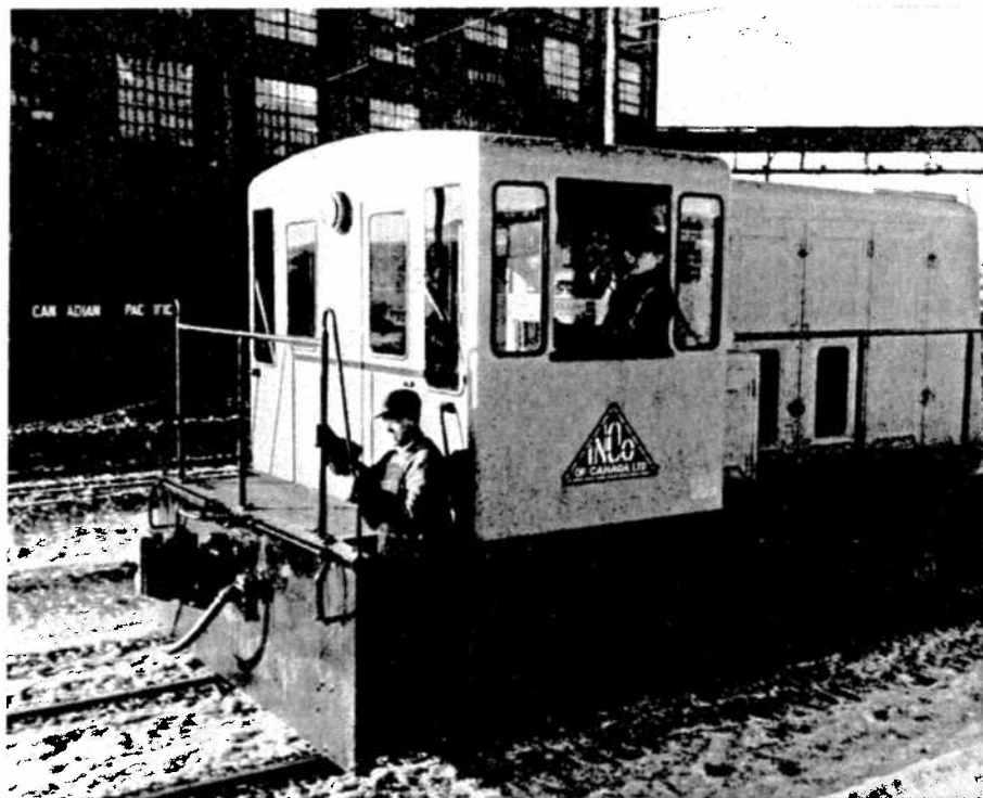
Seen operating the spanking new 35-ton diesel electric yard locomotive at the Copper Refinery are engineer Charlie Coulombe and his switchman, Guiseppe Saffi. Replacing the gasoline engine that had been in service since 1930, this new loco has the jump on all standard gauge rolling stock in the Refinery transportation system with its extra weight and 275 horsepower.
