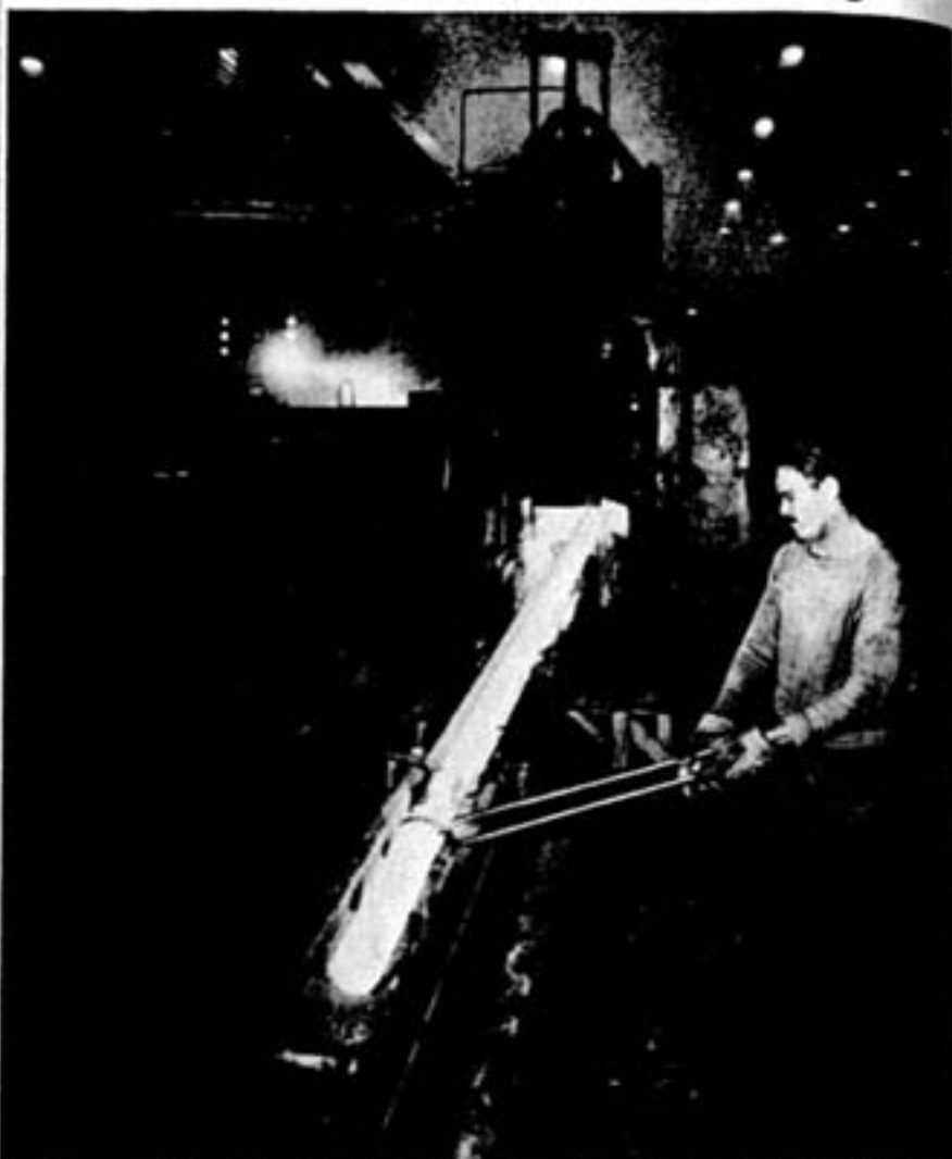
The new Inco high-nickel alloy Nionel is produced in all standard mill forms, including seamless condenser tubing, pipe and extruded tubing. Picture shows a length of Nionel pipe emerging from a hot extrusion press at the Inco works in Huntington, West Virginia.
