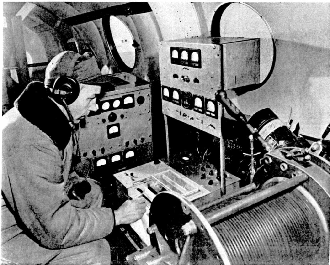
Here's what it's like in an aircraft equipped for an electro-magnetic survey. The operator, Vic Kanerva makes a notation on the recorder chart to assist the geophysicists in assessing the significance of the information picked up by the instruments. Opposite him is the receiver, and on his left is the transmitter which sends out the signal to the "bomb" towed beneath the plane on a 500-foot steel cable paid out from the winch in the immediate foreground.
