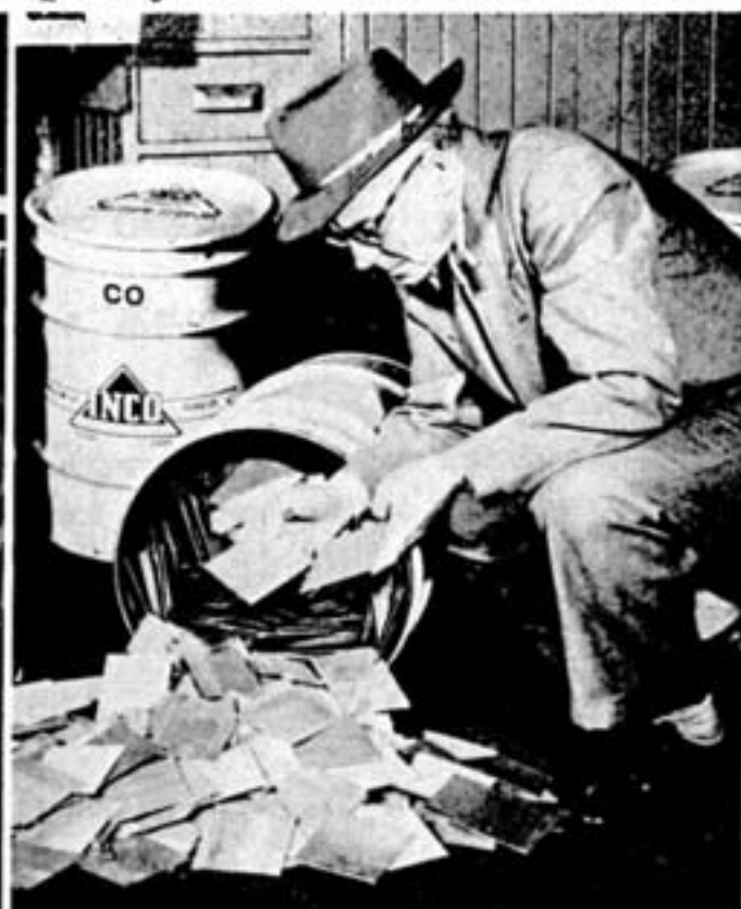
Donato Deluca, in the first of the above pictures, strips a sheet of cobalt from the stainless steel blank on which it has been electrolytically deposited at Inco's Port Colborne Refinery. In the second picture some of the first shipment of electrolytic cobalt from the Port Colborne Refinery is being inspected by R. C. McQuire, manager of Inco's Nickel Refining Division.
