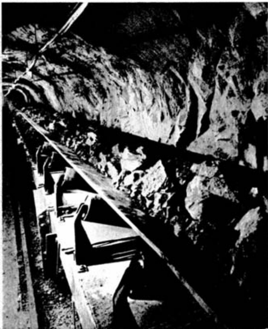
Inco's longest conveyor is underground on Creighton 30 level, carrying ore from No. 3 Shaft 1,820 feet to No. 7 Shaft for hoisting to the concentrator crushing section.
