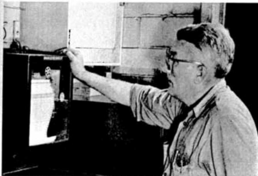
Aubrey Wright, foreman of the Cottrell plant, checks the temperature record. Gases must be kept hot to avoid condensation as they pass through the treater section.
