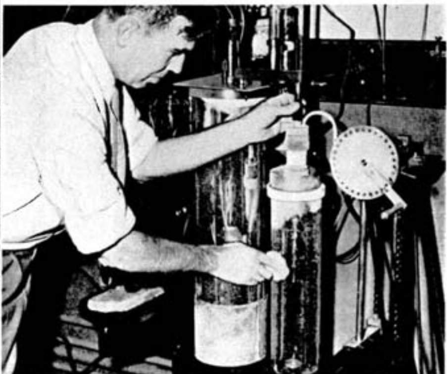
Designed to withstand internal pressure of 4,100 pounds per sq. in., a thick-walled Monel chamber stores helium which has been cooled in inner coils by liquid air and cold hydrogen vapors. The outer tank contains liquid hydrogen, which exposes the Monel chamber to temperatures below -435^{\circ}\text{F} . The helium is liquefied as it is valved out of this apparatus.
