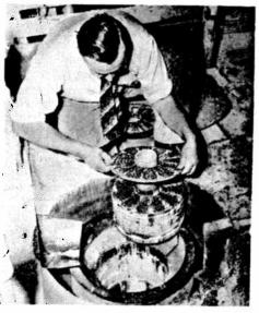
was found, however, that the coating was soon worn off by the abrasive clay, thus exposing the steel, which rusted and added further contamination by iron oxide. To overcome this condition pure nickel strip was substituted.
