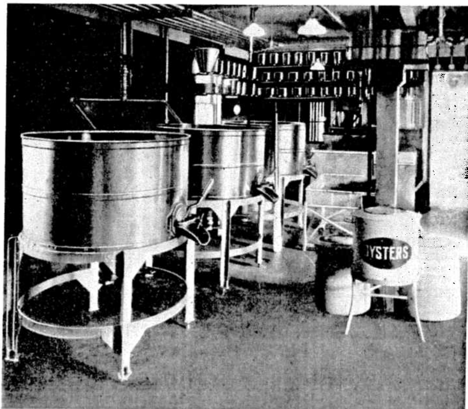
You'd think the last thing a fish would need would be a bath, but before oysters are packed they have to undergo a real "Saturday Night-er." These big Monel bath-tubs are used because the Monel is immune to chemical action and corrosion, and safeguards the oysters from contamination by rust and other impurities.
