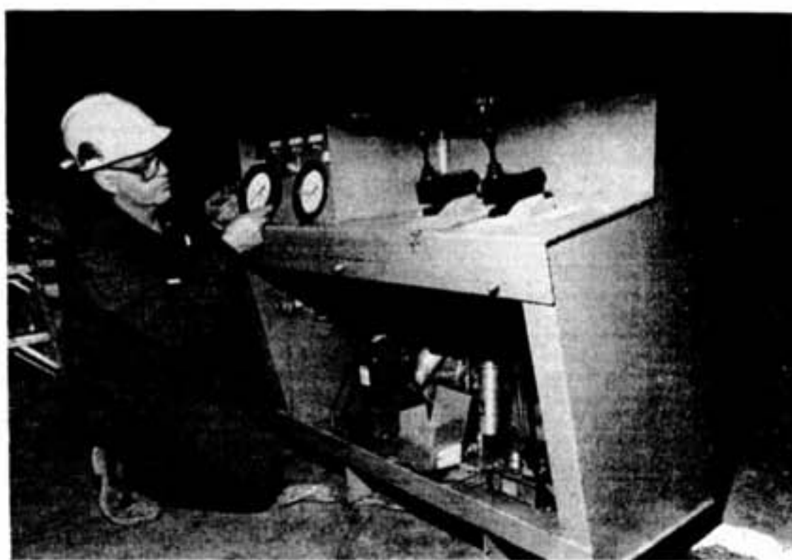
Rick Gagnon works on one of the new electrically-operated crusher consoles at Clarabelle Mill.
