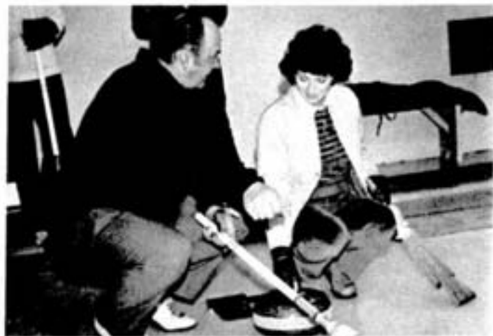
Machinists Mike Bauer and Clint Minor install internal plugs to regulate the circulation of cooling water through the holes drilled in the mould.
