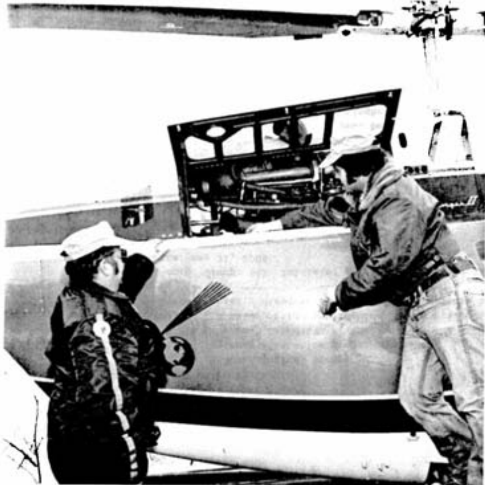
A stringent pre-flight check includes visual inspection of all major components. Here Len and Gary test the connection of hydraulic hoses in the engine compartment. It is interesting to note that the engine itself weighs less than 170 pounds.
