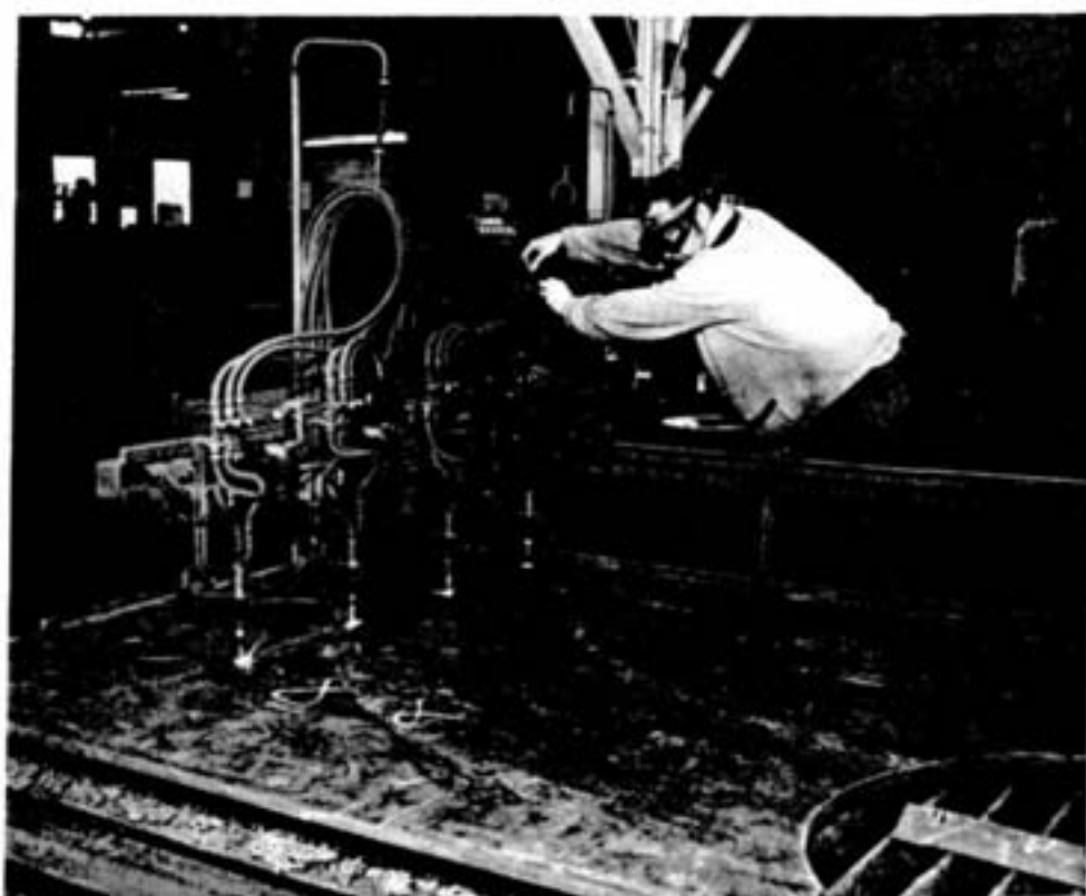
Gary Cresswell , plateworker 2nd class, is burning flanges with this newly-acquired automatic multi-cutting burning unit at the Copper Cliff plate shop. According to Art Oliver , fabrication shops co-ordinator, the new machine, equipped with four torches, is fully automated and works off an electric eye which follows a set pattern on the tracing table; it is the first unit of its type to be used at International Nickel.
