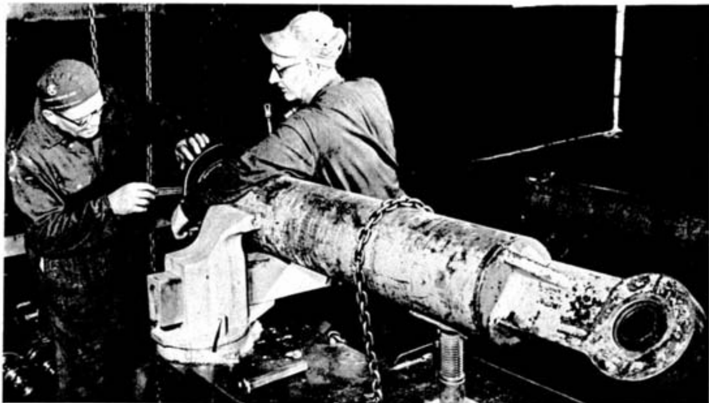
George Shepherd designed the cradle this ST4 dump cylinder is resting in. Joe Krugas and Eddie Sharp are tightening the cylinder's outer locknut.
