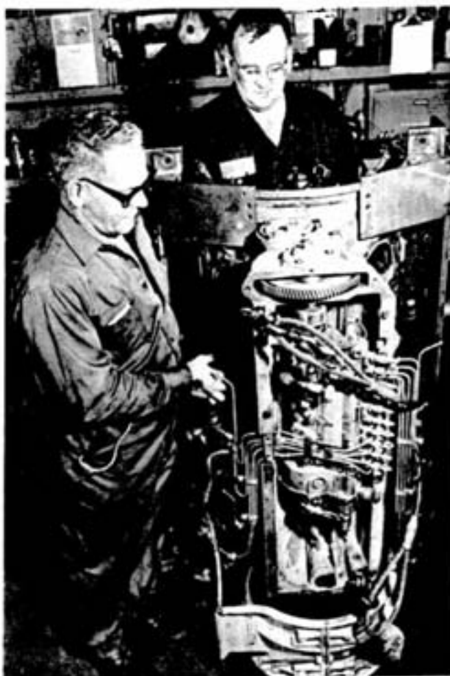
This 10 cylinder Deutz diesel was in the shop only three days. Burt Rush and Richard Lampman are replacing a cylinder in one of the special engine stands.
