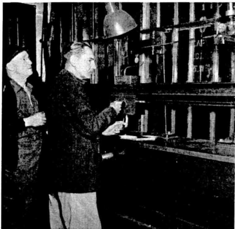
At the west scalehouse at Copper Cliff, while Henry Norris weighs in a car of ore on the big track scale, Eddie Saville checks an adjustment he has just made to the scale's recording device. Picture on the right shows Eddie at the Creighton mill, making a correction in the delicate mechanism of one of the four electrically controlled chronoflo scales that measure the feed to the grinding section.
