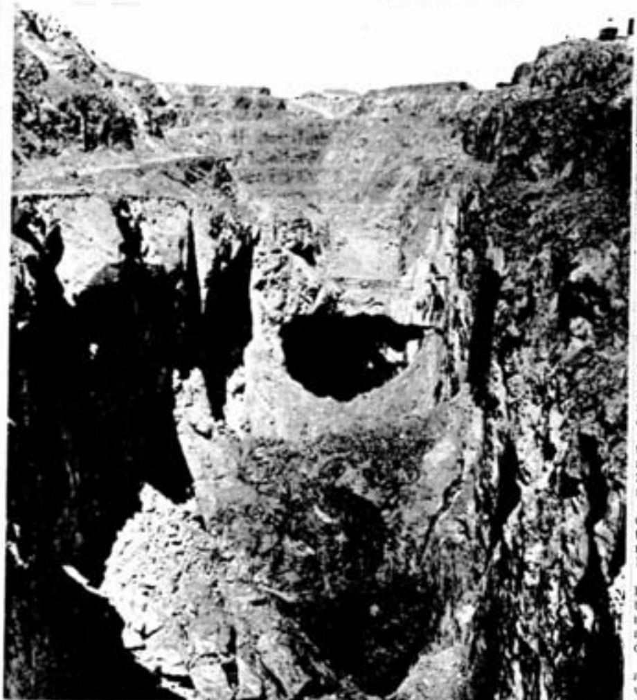
From the extreme south end of the Open Pit the camera looks down on underground mining operations, which have taken over in that section. The opening in the centre is the top of a huge blasthole slope which has been mined out from underground. Bridged above the slope is an inclusion of rock, about 230 feet long and some 175 feet at its deepest point, which will not be removed.
