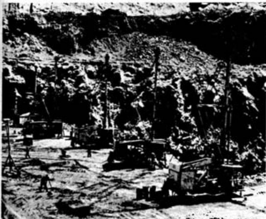
This closeup shows a battery of five churn drills pounding away at the stubborn ore as they sink a series of 9-inch holes in preparation for the next blast. Still another blast is in the making as the engineers make their survey. Weight of the churn drill tool string is over two tons, total weight of the drill is 25 tons. Churn drill holes are usually from 50 to 60 feet deep. The drilling rate is from 18 to 20 feet per shift.
